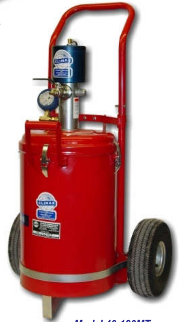
Model 40-120MT 5-Gallon - 40-lb. Pail 120:1 Ratio - 100 PSI Inlet Pressure Produces 12,000-lbs. Sealant Pressure
